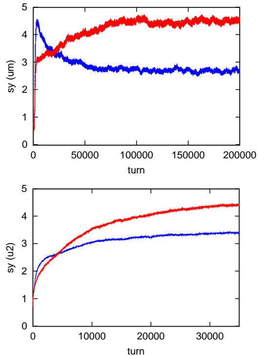
Figure 2: Evolution of vertical beam size given by the quasi-strong-strong simulation (upper) and the strong-strong simulation (lower). Red and blue lines depict evolution of positron and electron sizes, respectively.
