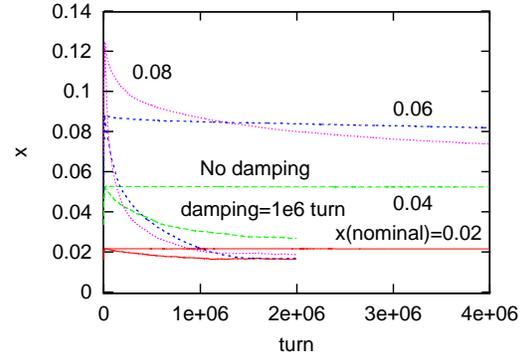
Figure 5: Evolution of the beam-beam parameter for very slow damping. Eight lines with four color depict the beam-beam parameters with/without radiation for four nominal beam-beam parameters, 0.02, 0.04, 0.06 and 0.08.
