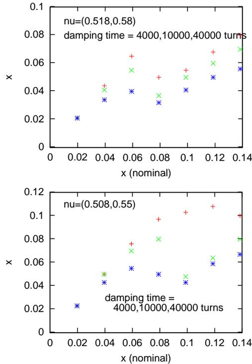
Figure 4: Beam-beam parameter for various damping time at two operating points. Red, green and blue points depict the beam-beam parameters for the radiation damping times of 4000, 10000 and 40000 turns, respectively.
