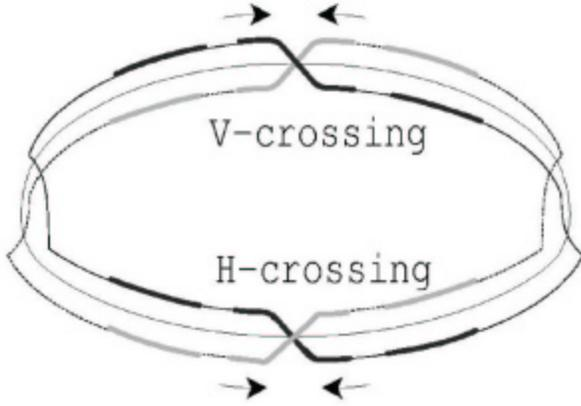
Figure 1: Schematic of a super-bunch hadron collider with alternating crossing at two collision points [6].
