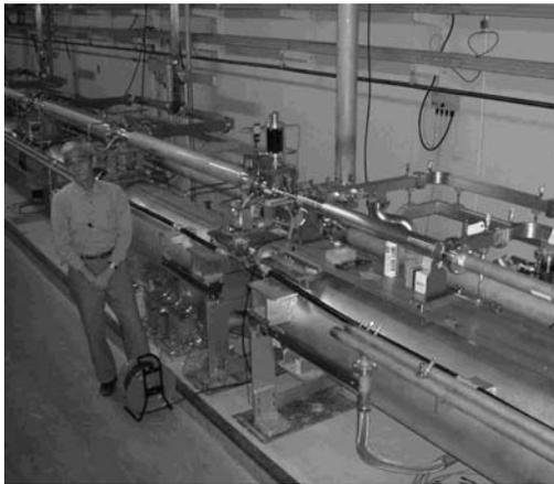
Figure 11 Accelerator guide installed at the #4-4 position
