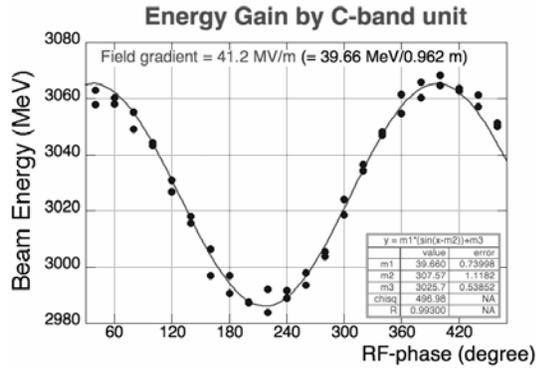
Figure 13 Energy gain measured by changing the RF phase when the output power from the klystron was 42 MW
