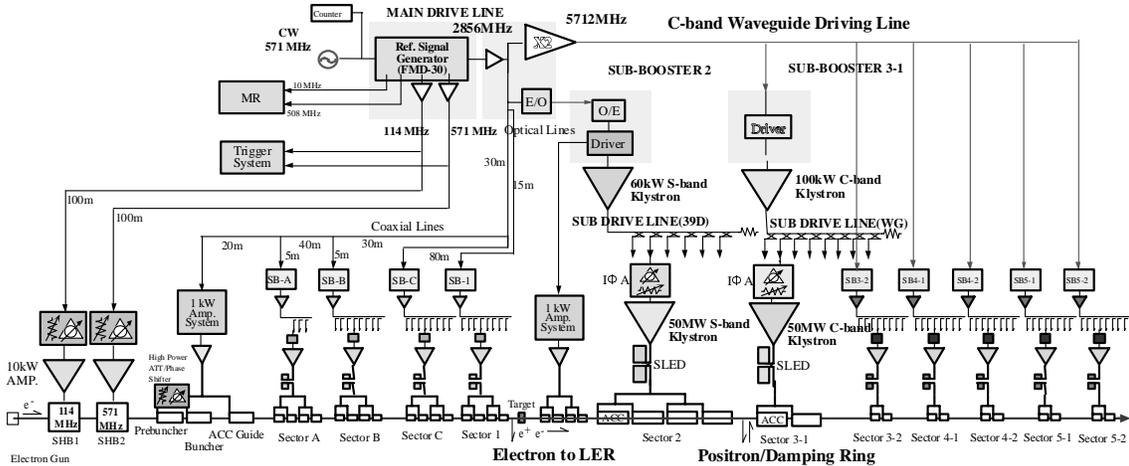
Figure 4 Block diagram of C-band system for SuperKEKB upgrade
