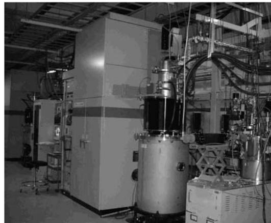
Figure 12 Modulator, 50 MW klystron assembly, and SB klystron installed in the klystron gallery
