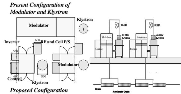
Figure 5 Comparison between the old and new modulators (left) and RF feeding scheme (right)
