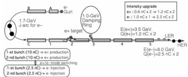
Figure 2 Simultaneous injection scheme using C-band system
