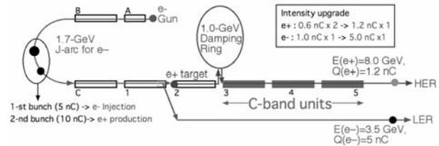
Figure 1 Proposed scheme using C-band system
