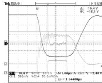
Figure 8 Waveforms: Voltage pulse (top), phase (second), current (third), and output RF (bottom). The horizontal scale is 1  $\mu$ s/div
