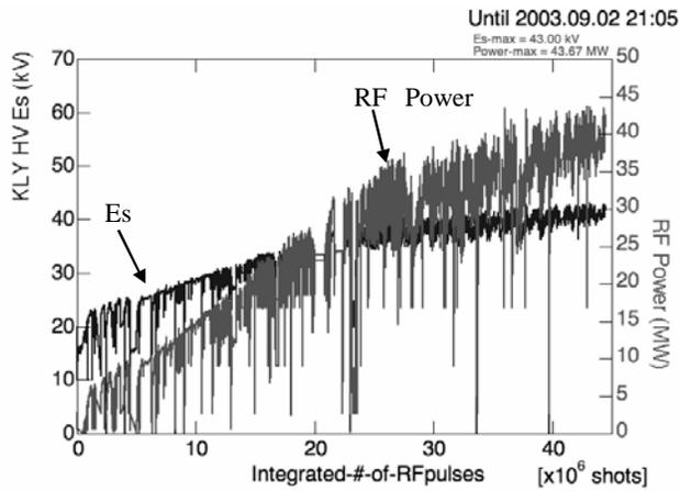
Figure 10 Processing history of the accelerator guide as a function of the RF pulse shot numbers
