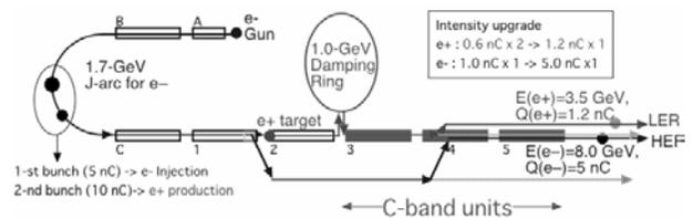
Figure 3 One of the possible schemes using a C-band system if there is no energy change
