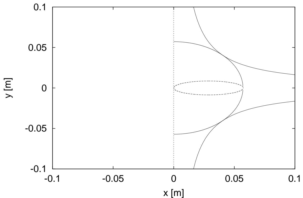
Synchrotron radiation fan (top view):
