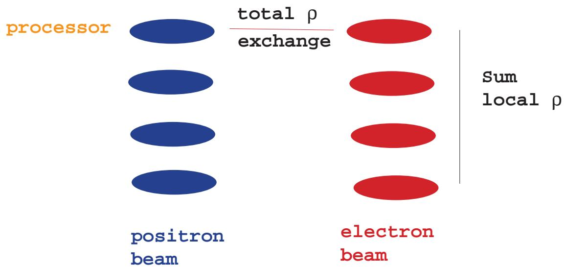
Macro particles are distributed on many processors. The processors are divided into two groups, one for positron beam and the other for electrons. The beam distribution on grid is summed within each group and then exchanged between the groups.
