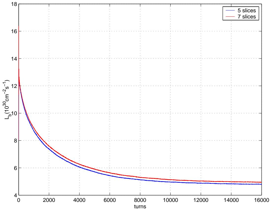
At peak intensities (1.6/1.22mA), simulated luminosity with 5 slices is  $4.812 \times 10^{30} \text{ cm}^{-2} \text{s}^{-1}$ . With 7 slices, we have  $4.954 \times 10^{30} \text{ cm}^{-2} \text{s}^{-1}$ . The difference is less than 3%.
