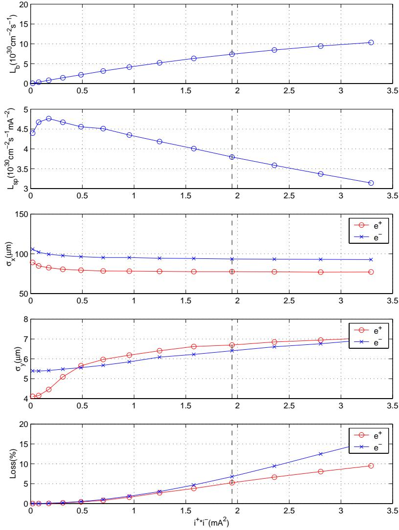
There are still room to increase the beam currents. Beams are matched at high currents in the vertical plane. There are more beam loss for electrons than positrons especially at higher currents. That can be a problem if the dynamic aperture is to large enough.
