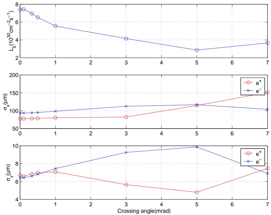
For  $\phi = \pm 3\text{mrad}$ , we see a degradation of luminosity by 43%. Similar results have been obtained by Ohmi and Tawada.
