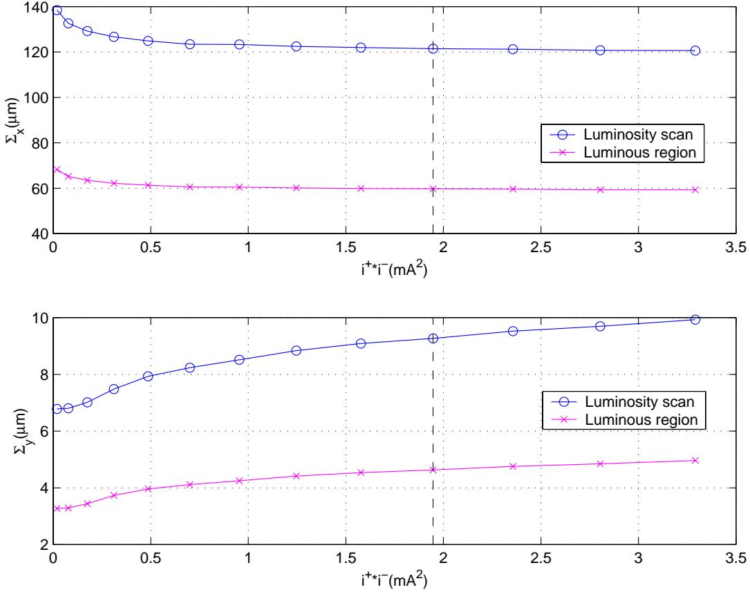
Based on the beam-beam scan at June 3, 2003, we have  $\Sigma_{max} = 161 \mu\text{m}$ ,  $\Sigma_{min} = 7.01 \mu\text{m}$ , and  $L_{sp} = 4.2 \times 10^{30} \text{ cm}^{-2} \text{ s}^{-1} \text{ mA}^{-2}$ . The luminous region seen by BaBar is  $\Sigma_x = 77 \mu\text{m}$ . The larger horizontal beam sizes in the experimental observations may be attributable to the huge beta beating in the High Energy Ring.
