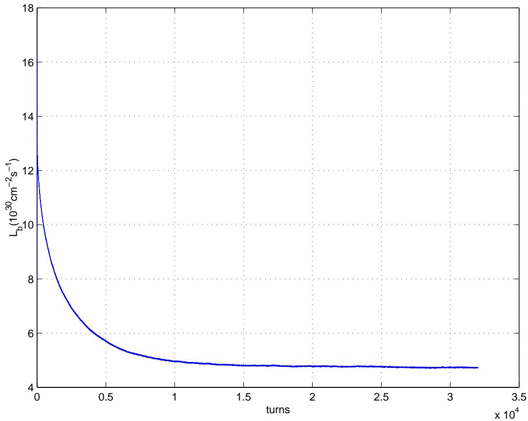
With interpolated slices, beams reach their equilibrium after three damping time.
