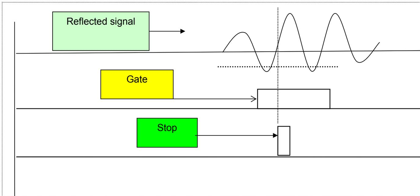
Time diagram of “zero level” comparator operation
