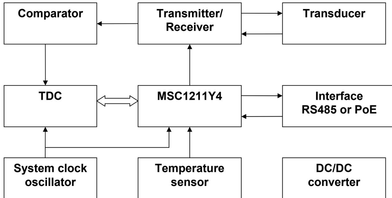
**Functional circuit diagram of the ULS electronics**
