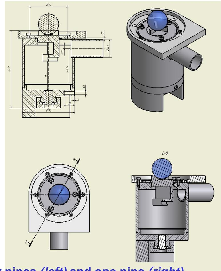
ULS design modifications: with two water pipes (left) and one pipe (right)
