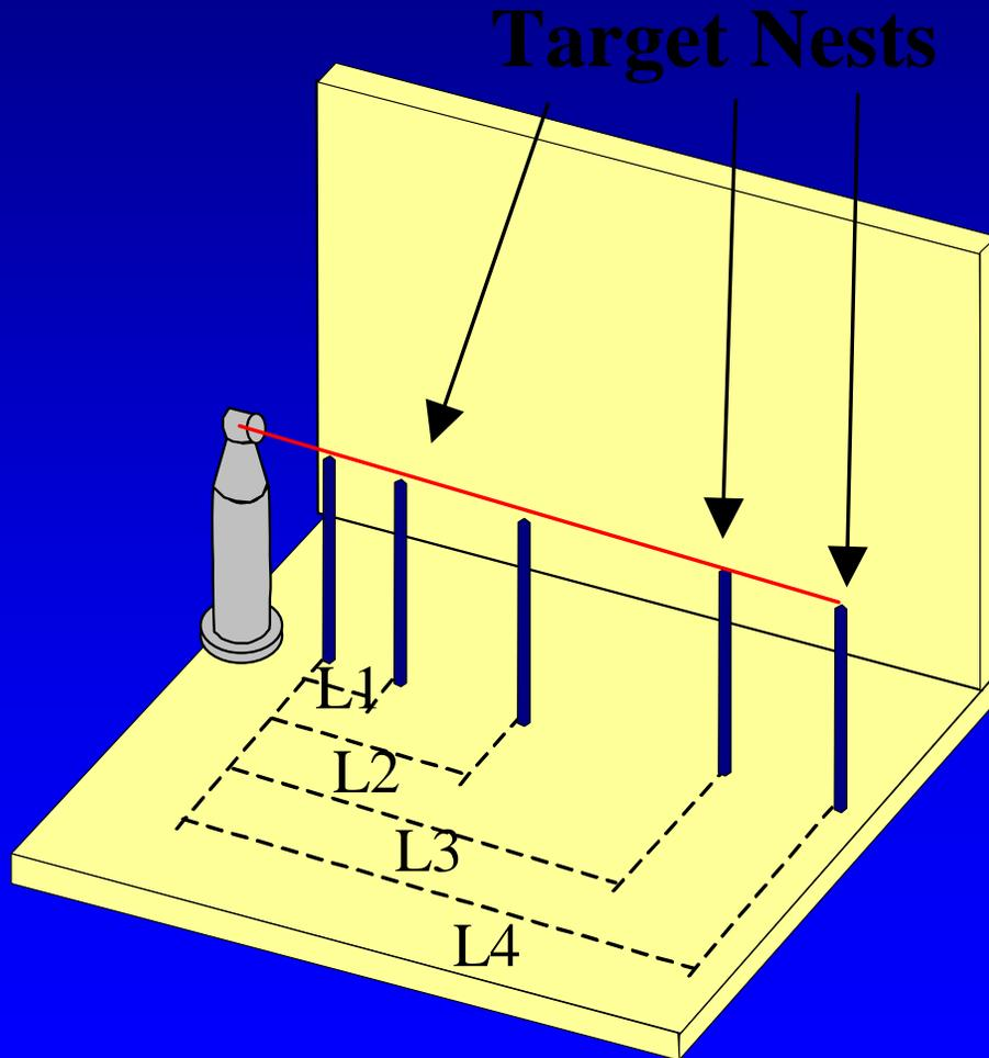
Four reference length measurements are required. Two additional user selected lengths shall be measured between the required maximum and minimum lengths ( $L1 \approx 6$  m and  $L4 \approx 26$  m)
