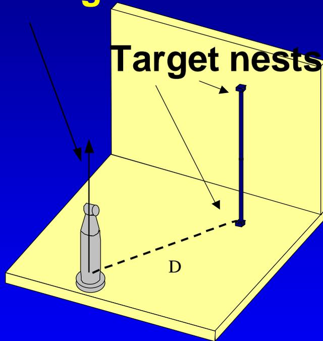
Reference length is measured in two positions a distance,  $D$ , from the tracker. In each position the tracker is rotated about the standing axis.  $D$  is between 2.3 and 6.3 meters in length.
