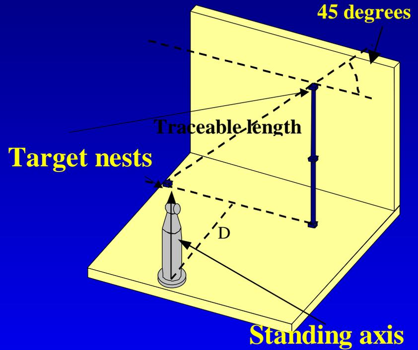
Test of combination of vertical and horizontal angle measurement capability
