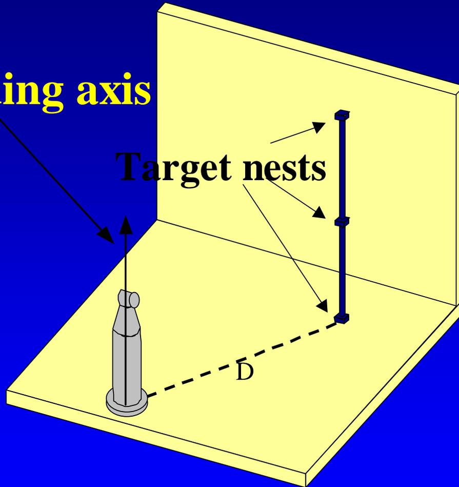
Reference lengths are measured in three positions a distance,  $D$ , from the tracker. In each position the tracker is rotated about the standing axis.  $D$  is between 1.5 and 6.3 meters in length.
