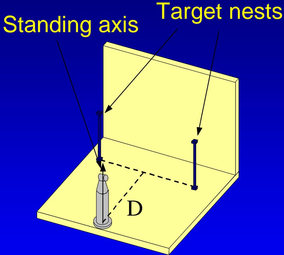
Reference length is measured in three positions a distance,  $D$ , from the tracker. In each position the tracker is rotated about the standing axis. The distance  $D$  is between 0.2 and 6.3 meters in length.
