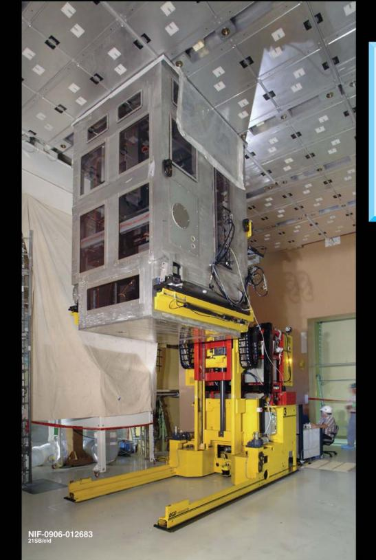
NIF architecture is based upon beam-path infrastructure containing kinematically-mounted Line-Replaceable Units (LRUs)
