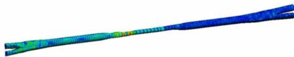
Figure 2. A localized mode identified in the PEP-II IR showing high loss (red) near the observed heating area.
