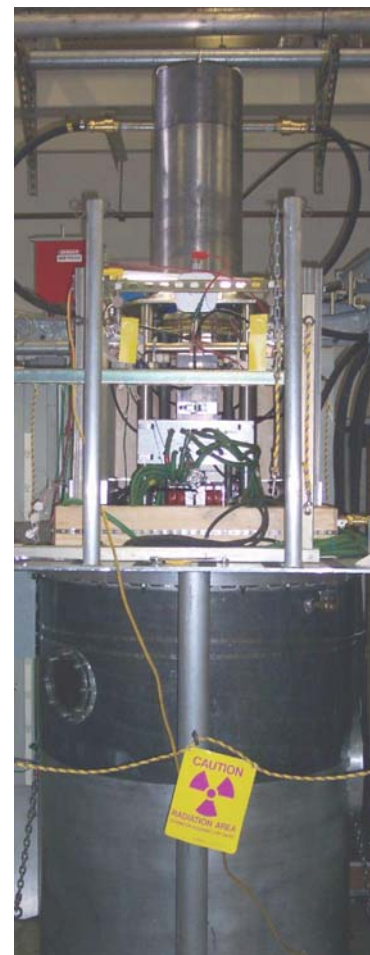
KEK PPM2 under test at SLAC
