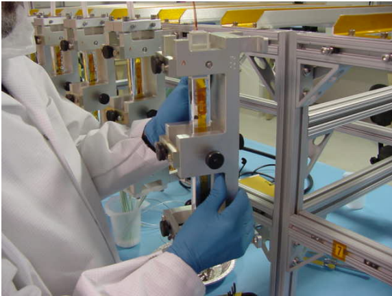
Calorimeter Crystal Detector (CDE) assembly at Swales Aerospace (1,728)
