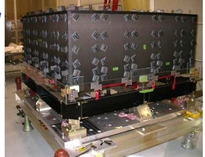
ACD Shell ready for vib test at GSFC
