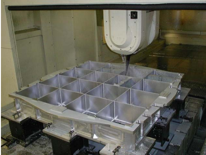
GRID Final Machining
