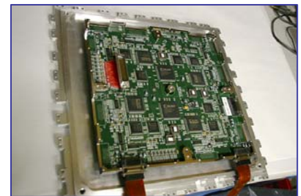
Tower Electronics Module (TEM)
