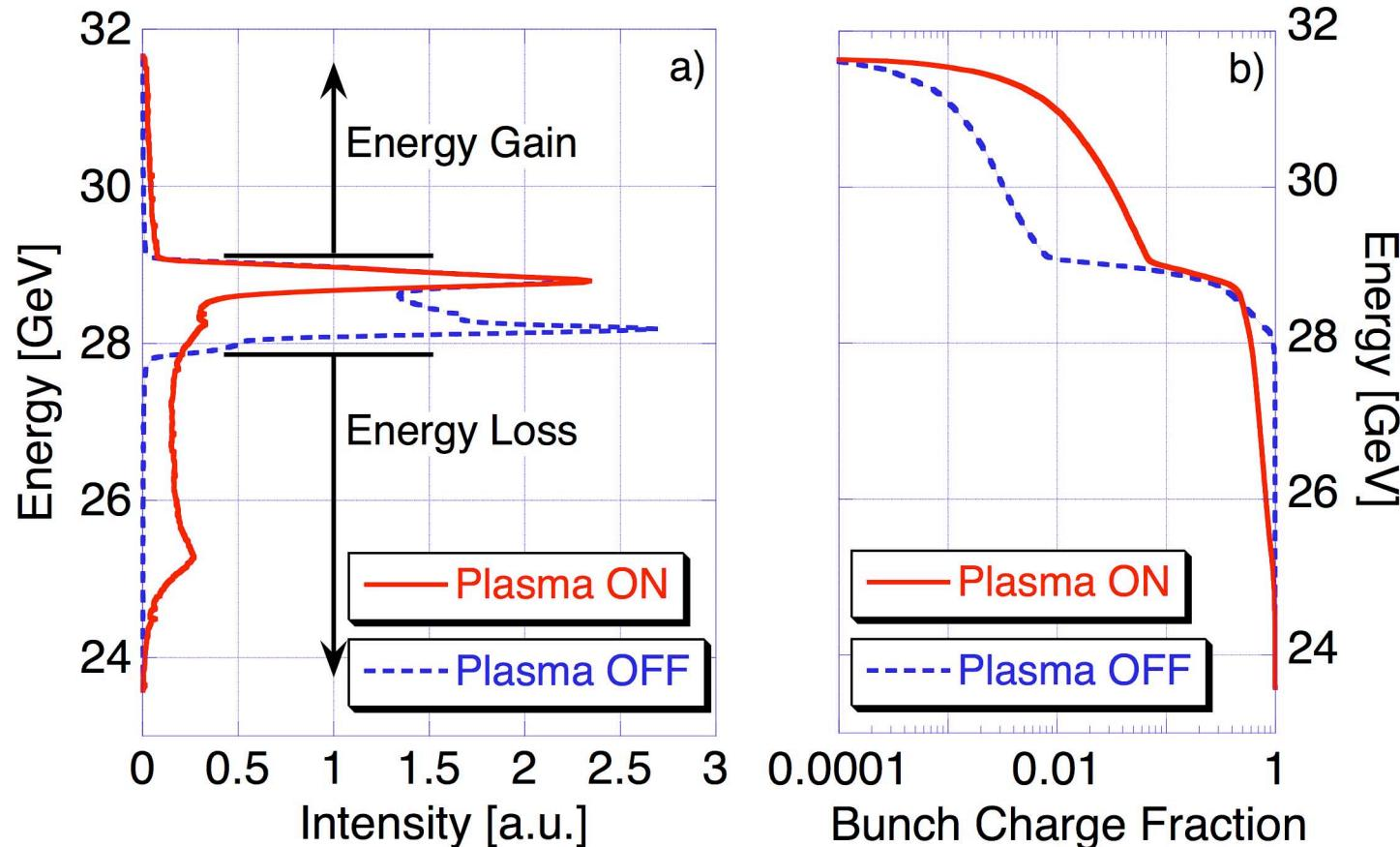
**Note:** The head of the bunch (25% of the highest energy electrons in the plasma off case) is below ionization threshold and not affected by the lithium vapor.
