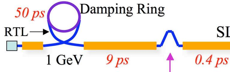
Add 12-meter chicane compressor in linac at 1/3-point (9 GeV)
