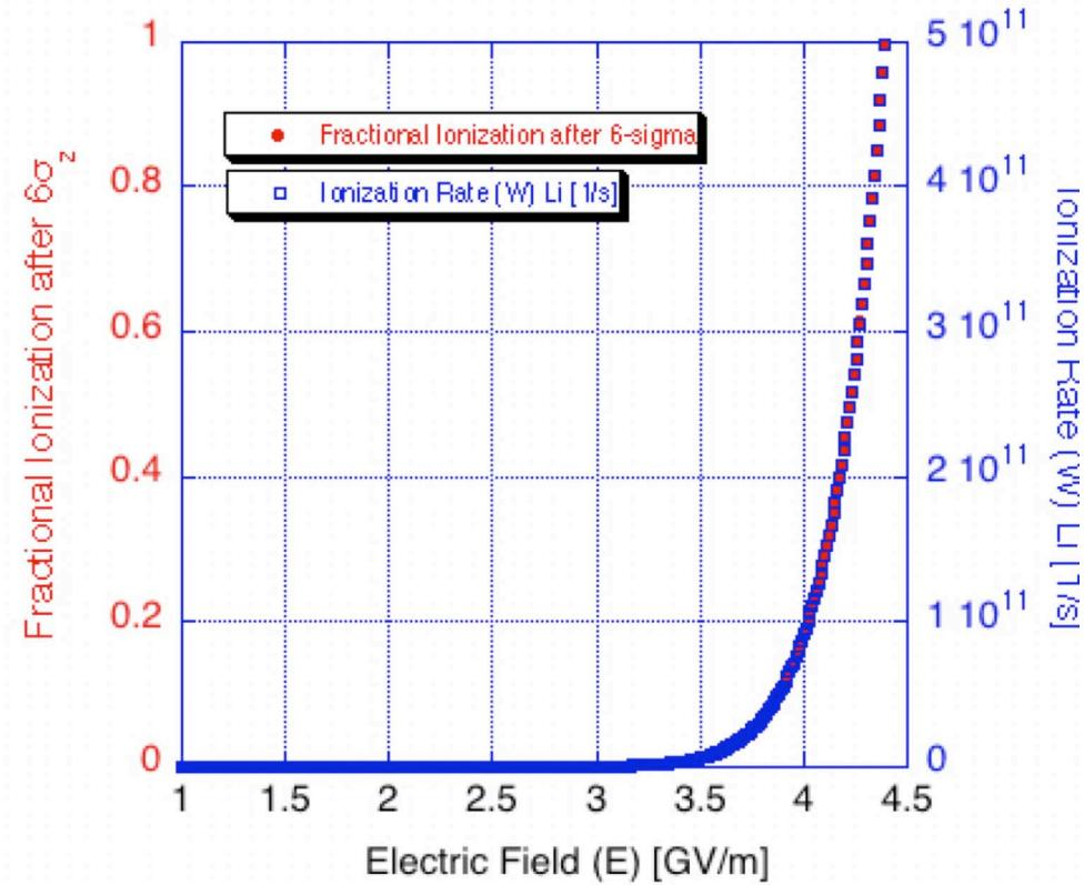
Space charge fields are high enough to field (tunnel) ionize - no laser!
