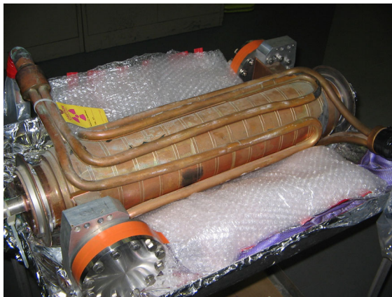
RF Deflector sections
