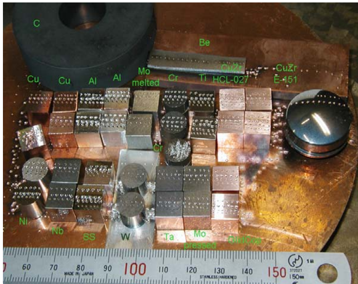
Profile of craters from 150 keV electron beam on 5 different metals: Tungsten, Molybdenum, Copper, Chromium, and Stainless Steel
