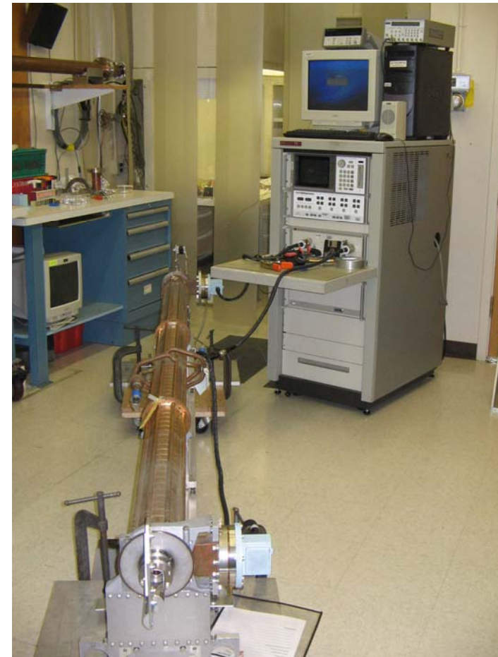
Horizontal microwave measurement and bead-pulling set-up.
