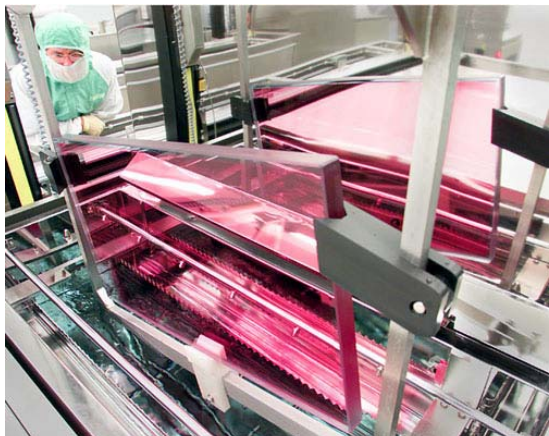
The Hoya Production II laser glass melting campaign was completed, yielding over 1700 amplifier slab blanks
