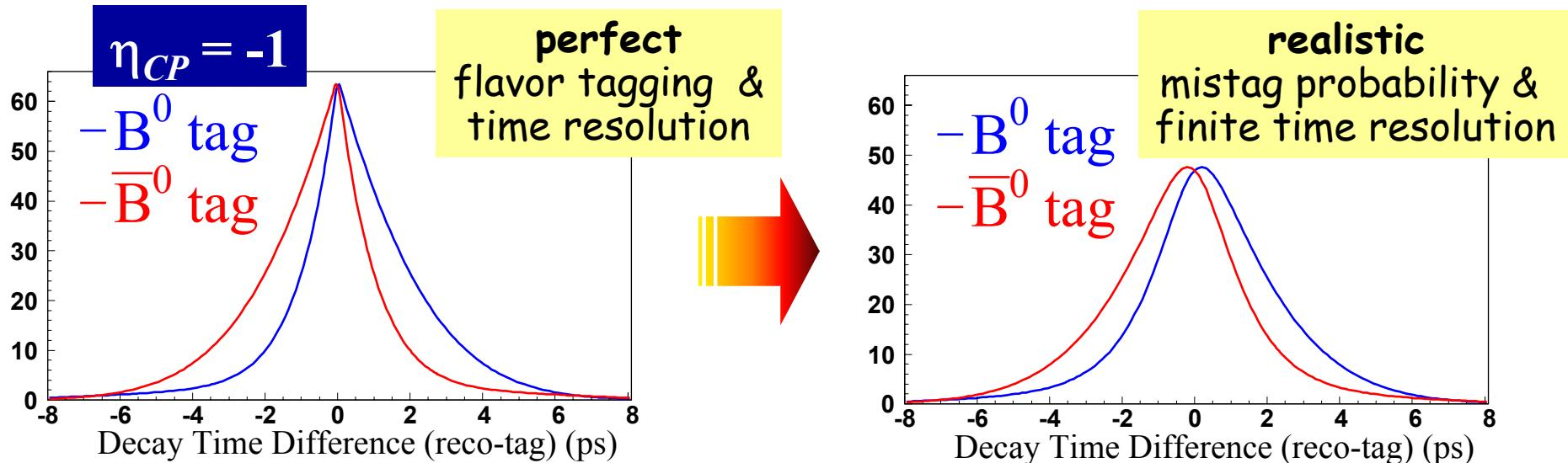
$$f_{CP,\pm}(\Delta t) \neq \left\{ \frac{e^{-|\Delta t|/\tau_B}}{4\tau_B} (1 \mp \eta_f (1 - 2\omega) \sin 2\beta \sin \Delta m_d \Delta t) \right\} \otimes R(\Delta t)$$
