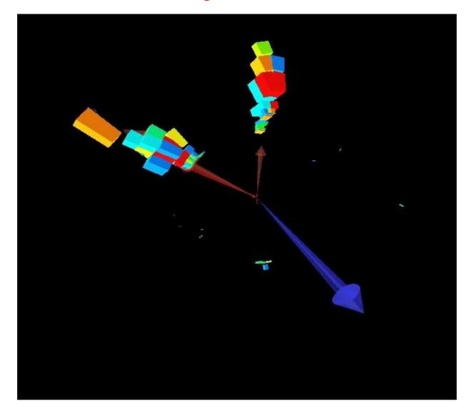
The colored boxes indicate energy deposits in the calorimeter. The blue arrow shows the direction & magnitude of MET.
