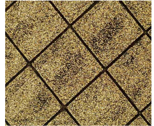
Detail of x-ray mask used for obtaining freestanding copper antiscatter grid
