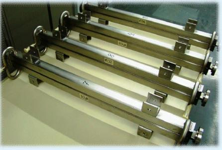
10 loads received from CINEL and VDL (material AISI316LN)
