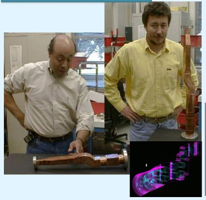
H10 -> H01 mode converter CERN design (needed for PETS on-off)
