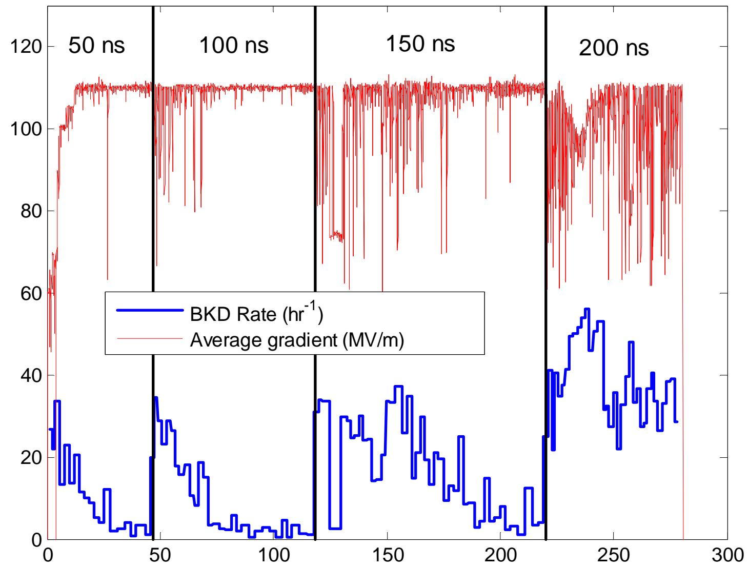
Comparison of current BDR rate (blue circle) with the rate curves from the First SLAC T18 structure at different processing times
