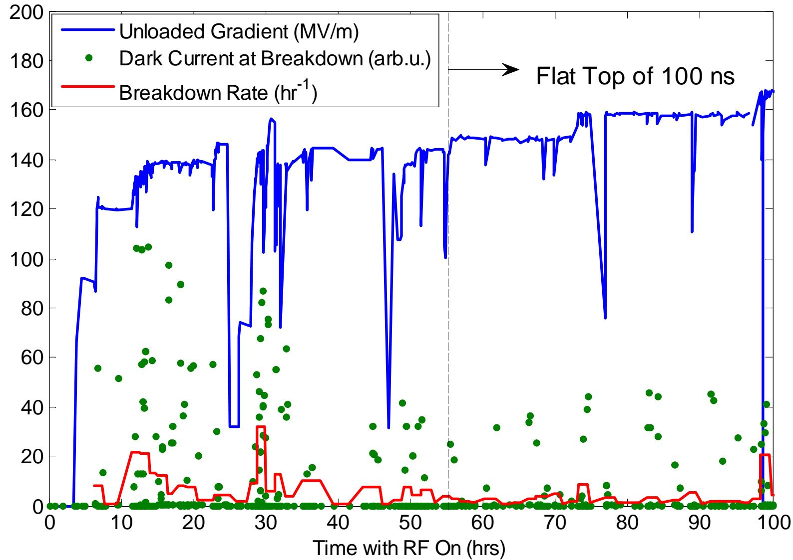
Detect breakdown from the large ( $> 0.8$  on above scale) current produced<sup>6</sup>
