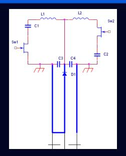
A simplified circuit to pump of the SLIM cell
