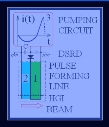
A presence of 100 MV/m field in the cell is only for 2 nsec. The rest of time the DSRD switch keeps gradient at zero level.
