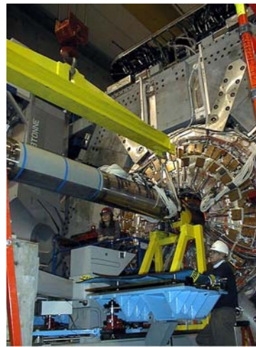
MN_129 ST 30: Setting Support Tube on Insertion Beam Hook 04/08/99
