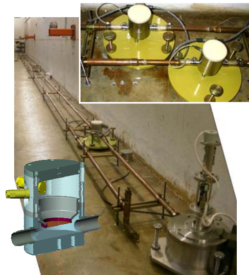
Figure 2: Hydrostatic Level System installed in the alignment laboratory at SLAC for NLC slow ground motion studies. The HLS sensors from this system were installed at PEP-II IR. The test device shown in the right hand corner allowed controllable micrometer variation of the water level, for calibration tests and water dynamics study. An insert in the left bottom corner shows cross-section of the sensor.
