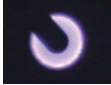
Figure 14: An example of the pictures of the multipactoring discharge in the coaxial line WX77D of the coupler.
