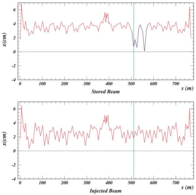
Wall clearances for Stored and Injected electron beams around CESR.
