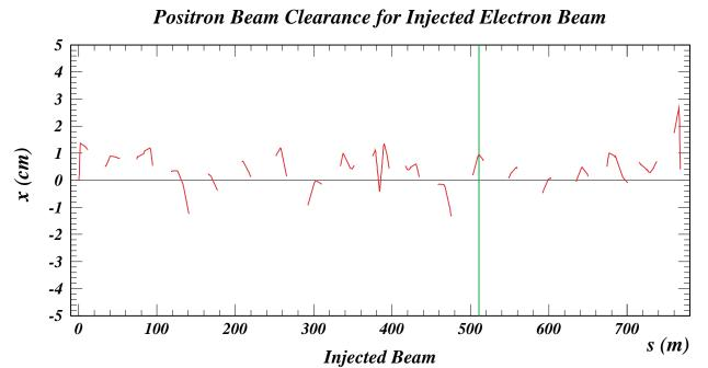
Clearance between the stored positron beam and the injected electrons.
