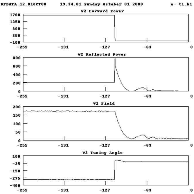
Beam Dump - RF Turns Off & Beam spirals to hit inside of vacuum chamber Causes Beam Induced RF Power as seen in the Reflected Power Signal (no Quench)
