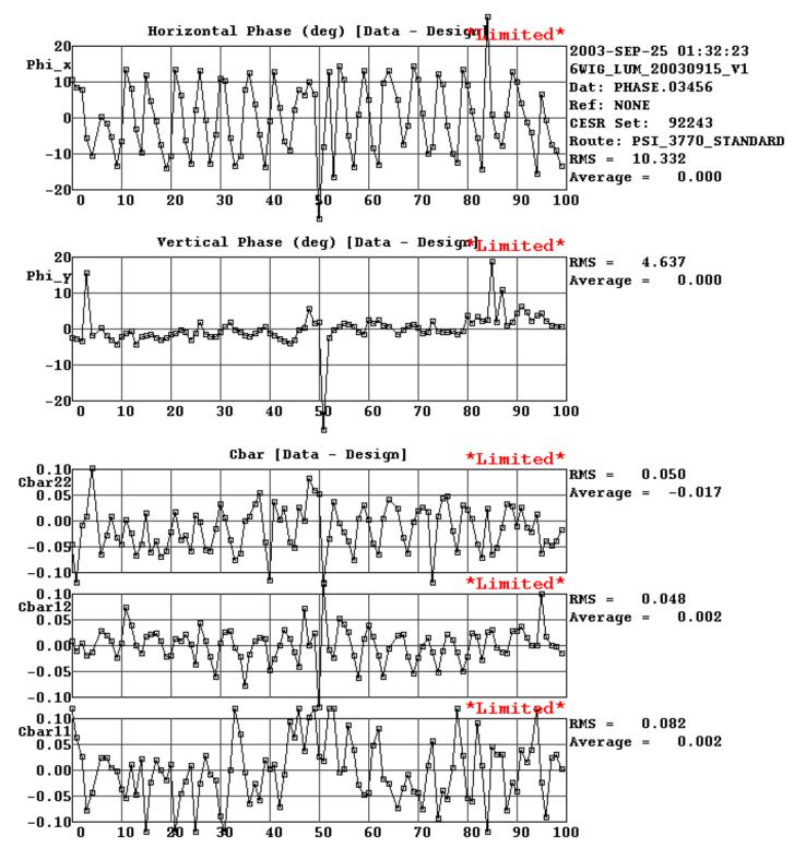
Betatron Phase Advance Error & Coupling Matrix Error
