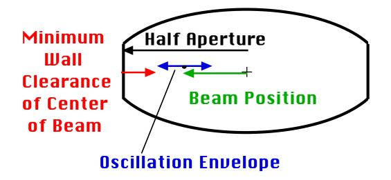
5. Determine any static or transient closed orbit distortion for stored beam or injected beam => Beam Position
