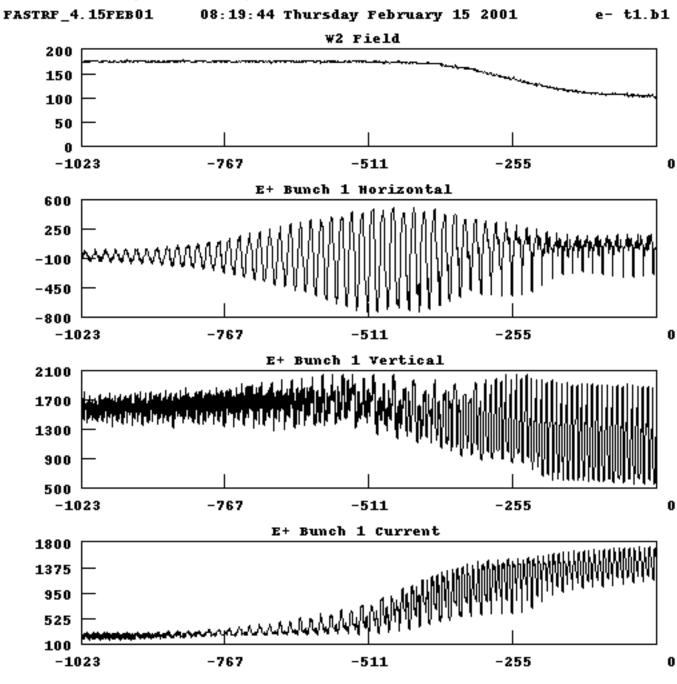
Positron beam became unstable longitudinally causing beam loss
