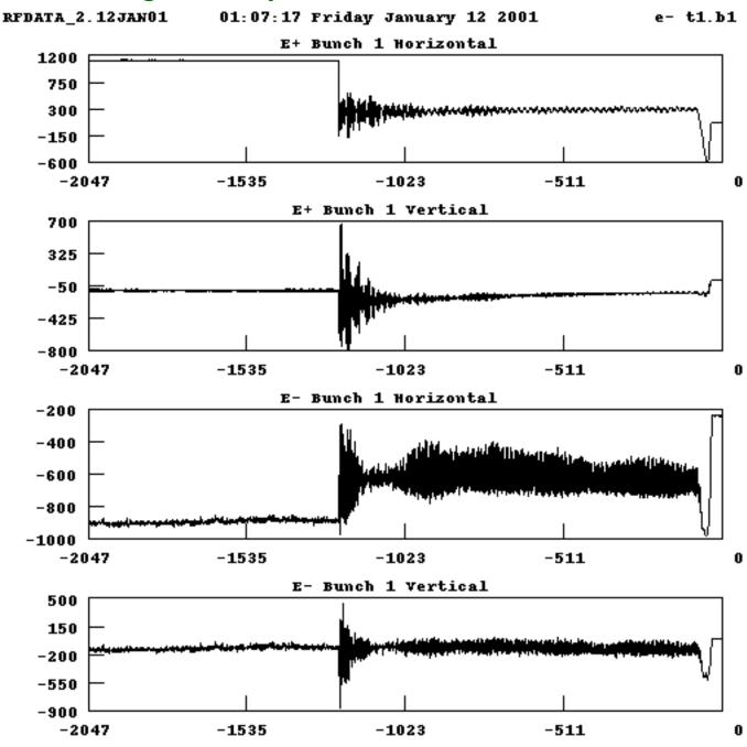
Horizontal Separator Trip causing beam to become unstable horizontally
