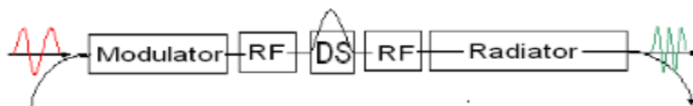
Figure 2: Dedicated scheme for the tuneable HGHG FEL RF sections are located before and after dispersive section locally providing the energy chirp required for the wavelength compression.
