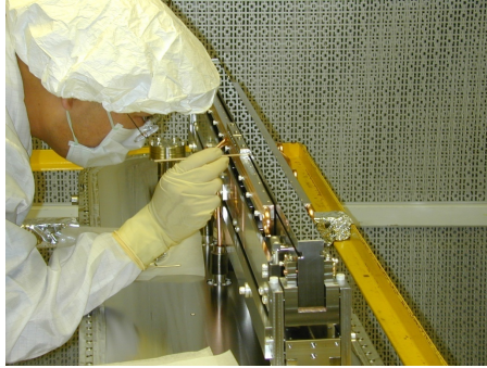
above: 1.0m Si flat, side-cooled M0 mirror employed for beam collimation
