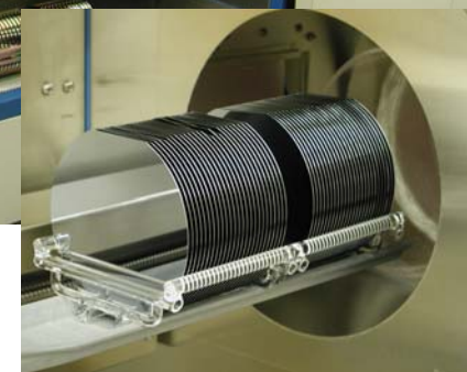
Atmospheric and low pressure chemical vapor deposition furnaces
