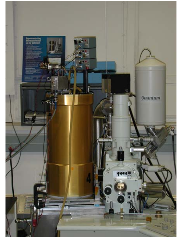
ADR and cryogen vessels mounted on SEM
