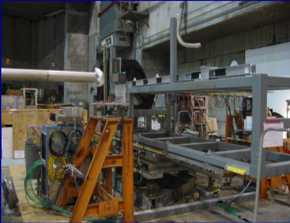
Setup in End Station A: movable bar support and hodoscope
