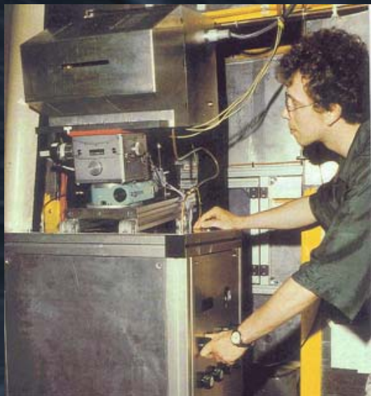
Detector HASYLAB Segmented double line ionization chamber
