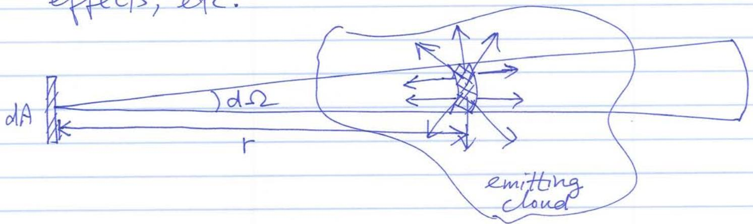
The idea is that every differential volume element of the cloud is emitting radiation isotropically. This is characterized by the emissivity  $q = q(\vec{r})$ , which varies throughout the cloud, and has units [volume<sup>-1</sup> time<sup>-1</sup>].
